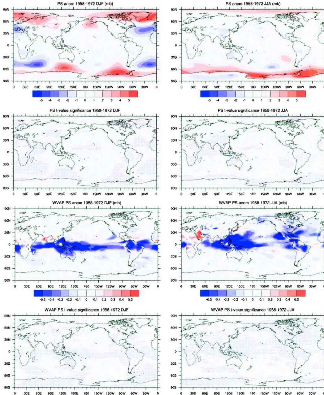
FIG. 6. Differences in means of (top four panels)  $p_s$  and (bottom four panels)  $p_w$  for 1958–72 compared to 1979–2001 in hPa (top in each group) and as  $t$  values (lower panels) for (left) DJF and (right) JJA. The latter have blue shading for significance at the 5% level and pink shading at the 10% level assuming one independent value per year.
