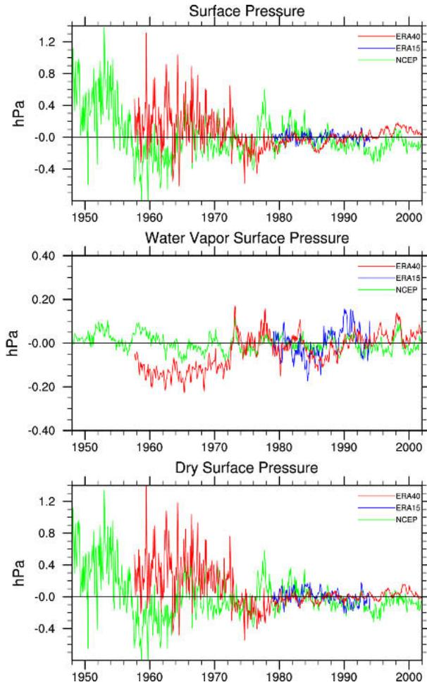
FIG. 2. Time series of global mean surface pressure anomalies relative to 1979–2001 for (top) the total  $p_s$ , and contributions from (middle) water vapor  $p_w$  and (bottom) dry air  $p_d$  for three re-analyses from ERA-40 (red), ERA-15 (blue), and NCEP–NCAR (green) in hPa. Note the amplified vertical scale of the middle panel.
