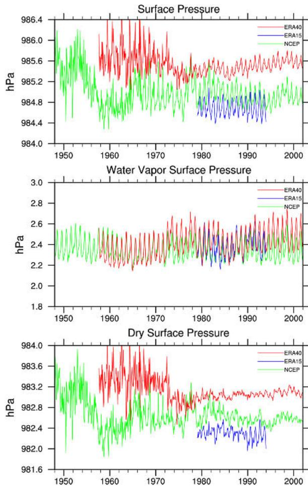
FIG. 1. Time series of global mean surface pressures for (top) the total  $p_s$ , and contributions from (middle) water vapor  $p_w$  and (bottom) dry air  $p_d$  for three different reanalyses from ERA-40 (red), ERA-15 (blue), and NCEP-NCAR (green) in hPa. (middle) The vertical scale is magnified compared to that of the (top) and (bottom).
