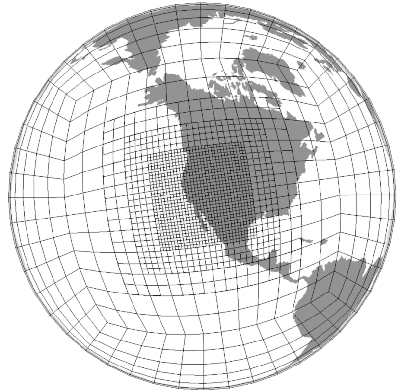
Figure: A cubed-sphere refinement patch over California.
