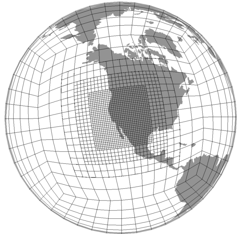
Figure: A cubed-sphere refinement patch over California.
