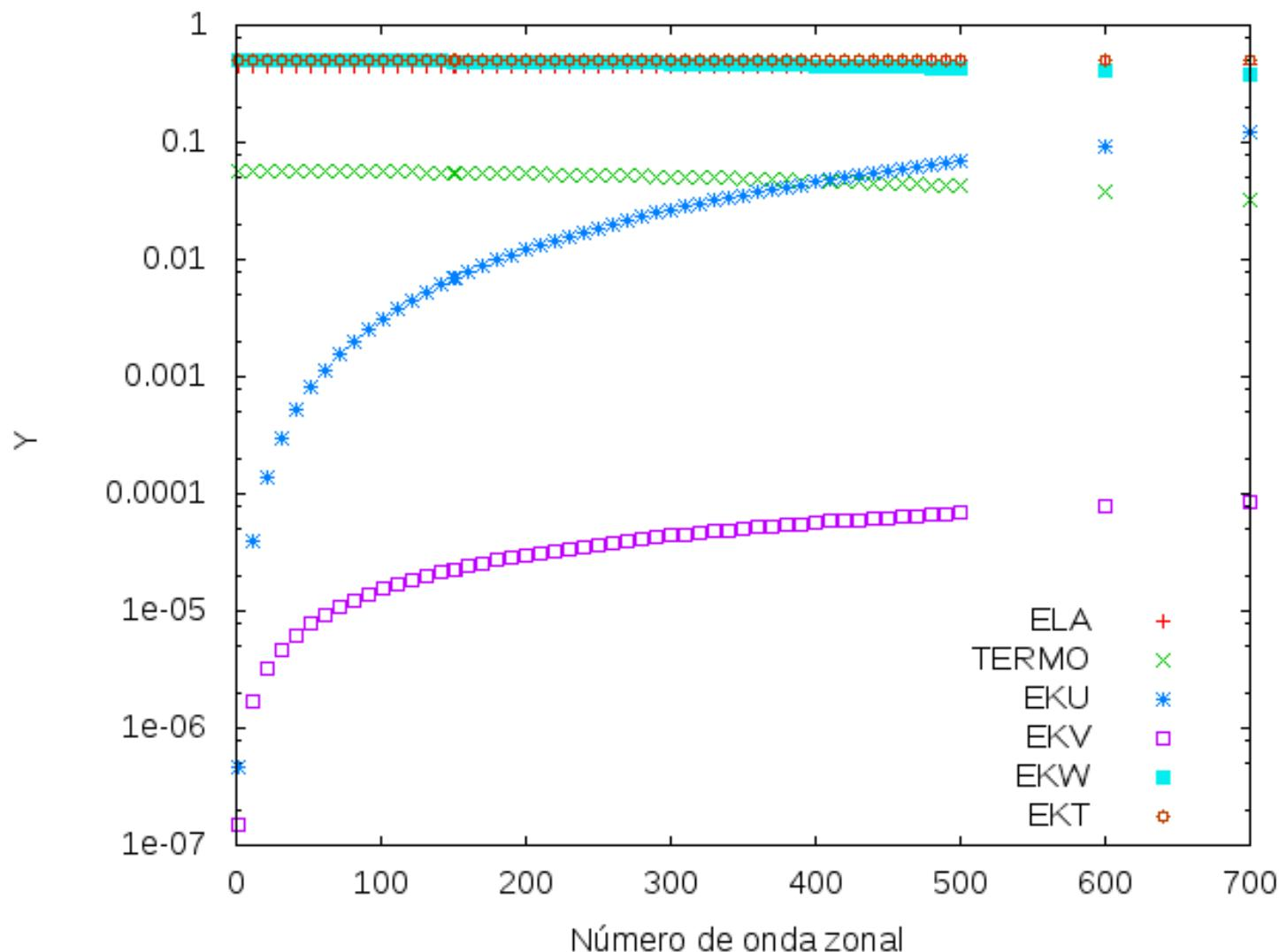
Energetics of eastward inertio-acoustic modes with meridional index  $l = 0$  and  $k = 1$ . Each energy type is normalized by total energy.
