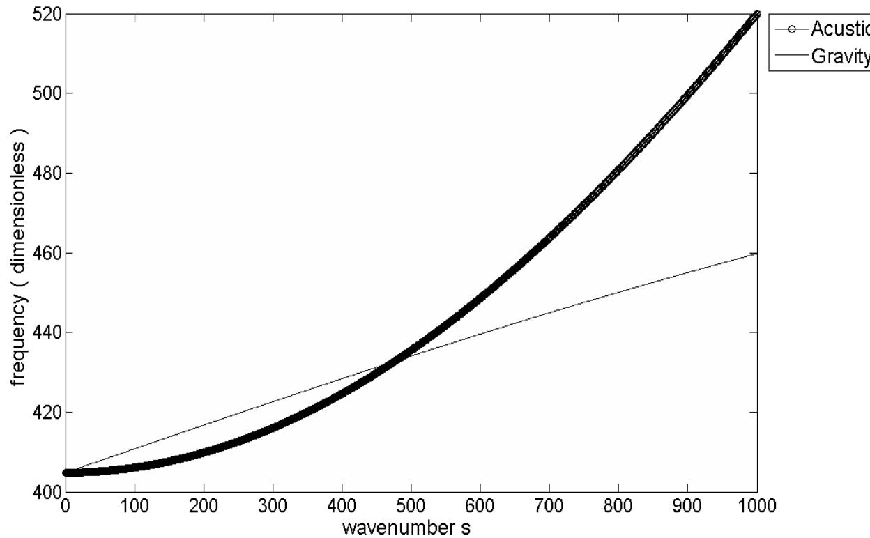
Determination of a resonant triad involving a long inertio-acoustic, a short acoustic mode and a short gravity mode. The acoustic modes have  $k = 1$  vertical structure, while the gravity mode has a  $k = 2$  vertical structure.
