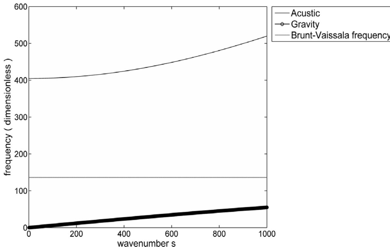
Dispersion curves for acoustic and gravity modes for  $l = 0$ ,  $k = 1$ , and symmetric about the equator.
