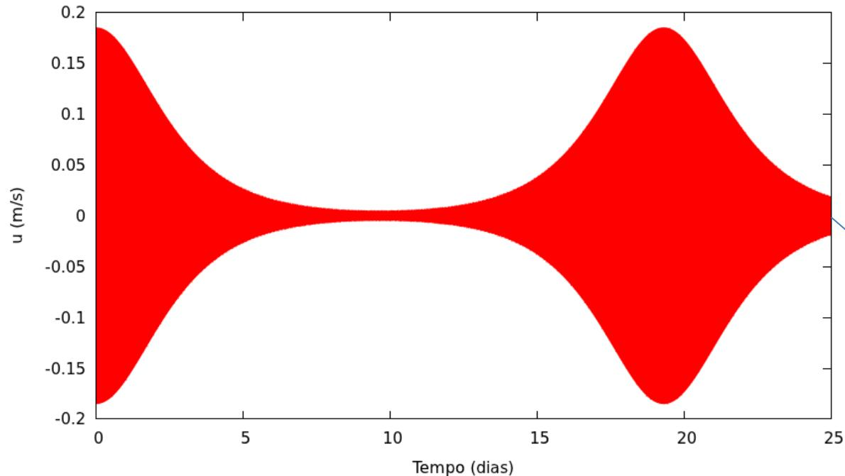
zonal velocity at  $\varphi = 0^\circ$  and  $z = 4.5\text{Km}$
