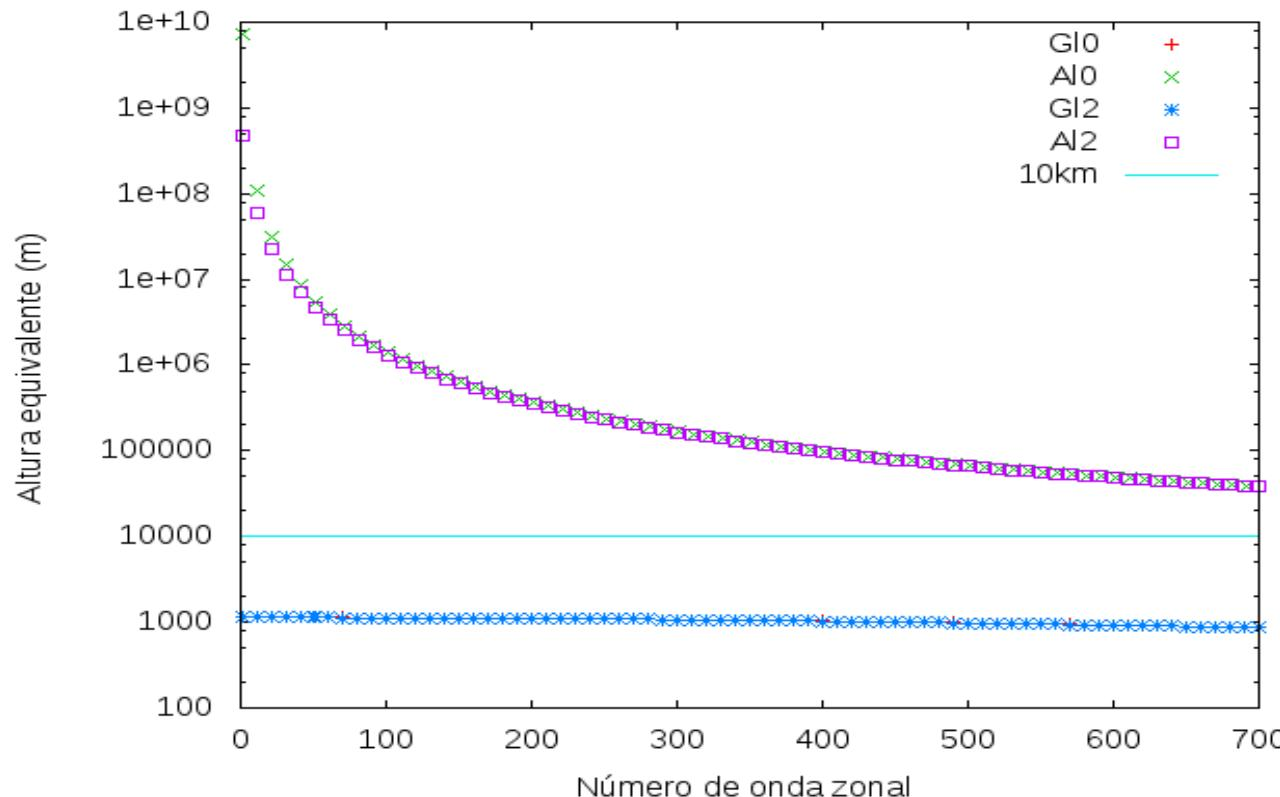
Equivalent heights  $H_e$  for acoustic and gravity modes for  $l = 0$ ,  $k = 1$ , and symmetric about the equator.
